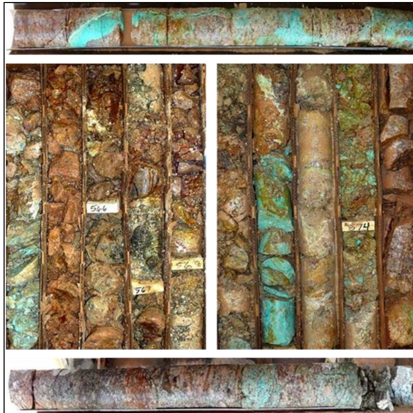
Figure 7-5: Florence Copper Drill Core showing granodiorite with bluish-green chrysocolla replacing clay-altered feldspars and in vein formation
