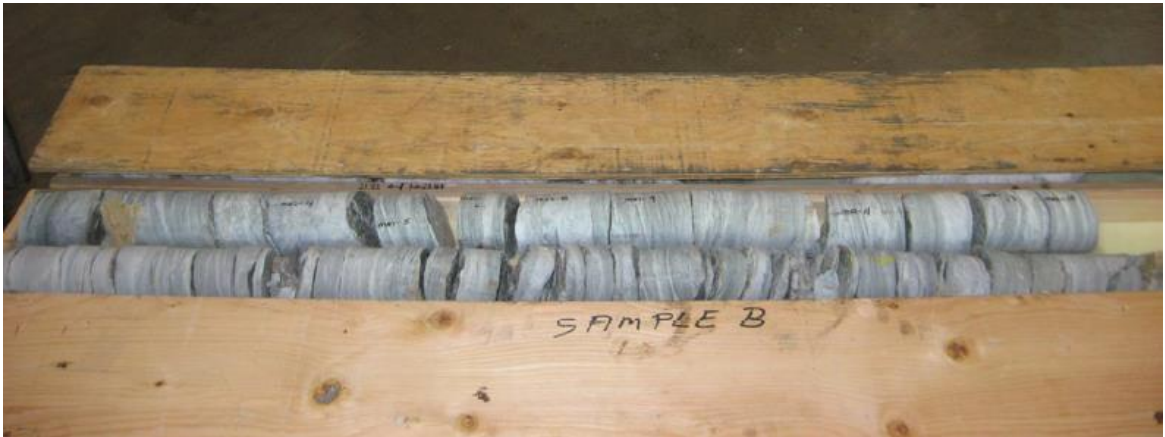
Figure 13-4: Platey Breakage Example on Core Sample B
